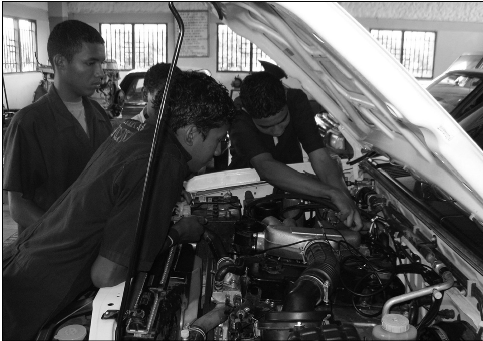
Image 3 CEVER students adapt a regular diesel engine to the direct use of PPO from processed Jatropha seeds
